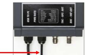
The most common connection to a dedicated chart plotter is to take the NMEA Output (Orange+ and Brown –) from the CLB1000 Transponder and to connect it to a free NMEA Input on the plotter. You must then tell the chart plotter that AIS data is connected to this port and set the baud rate to 38,400 Baud – the standard speed for AIS data. Consult the instruction manual supplied with your Chart Plotter to understand how this is configured.
